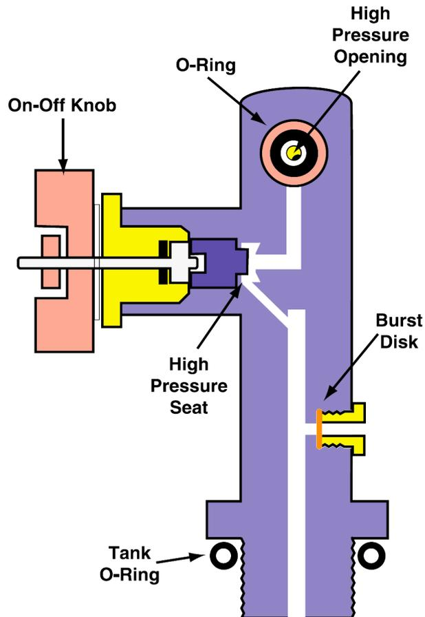
K-valves will either have a yoke fitting or a DIN fitting for the tank opening. This is for the different designs of first stages on scuba regulators. DIN screws into the tank valve.
